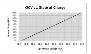
The graph shows that a healthy, fully charged NSB automotive and marine battery will have an OCV of approximately 13.0 V.
