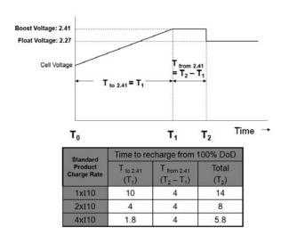
The table above shows the time needed to recharge following a 100% DOD cycle,
